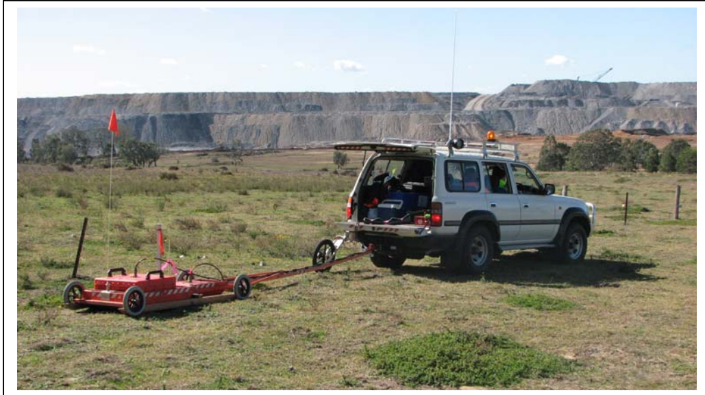
Figure 3: GPR investigation at Warkworth Mine in August 2007. Dual frequency antennae (200 MHz and 400 MHz) were used during the investigation and provided high quality data. It is proposed to use a similar set up for this investigation.
