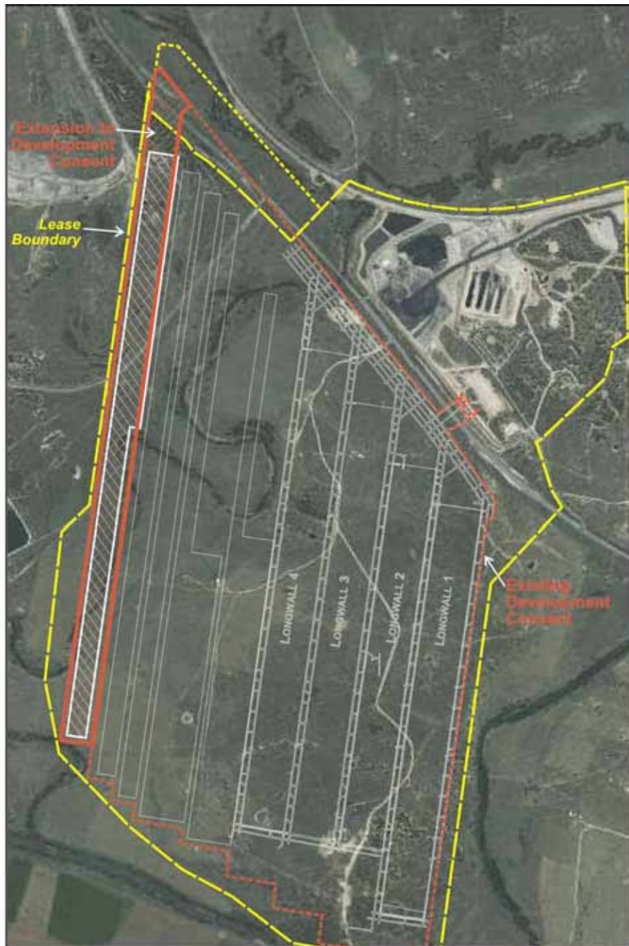
Figure 2 Longwall layout superimposed onto aerial photograph.
