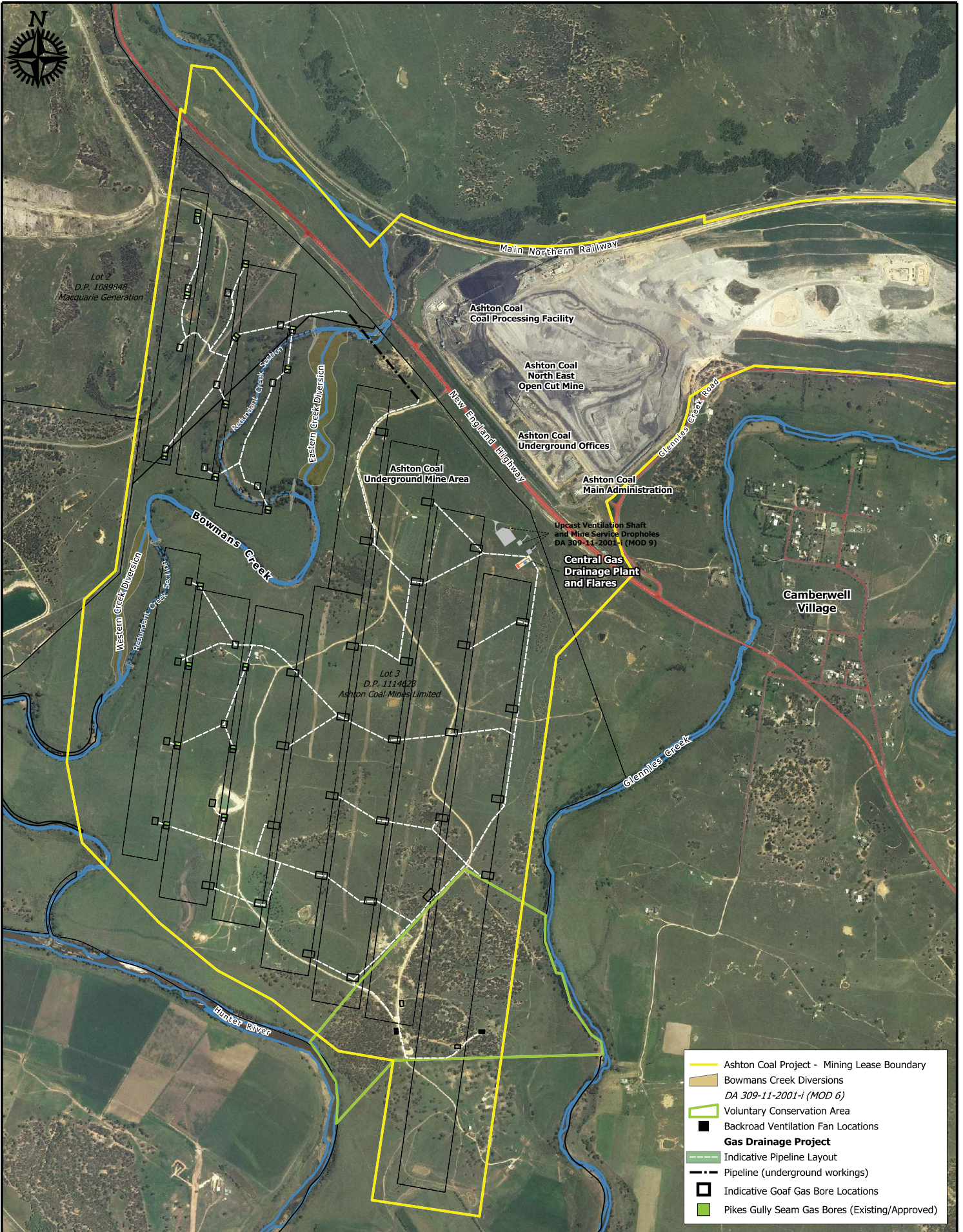
Indicative Goaf Gas Drainage Network
