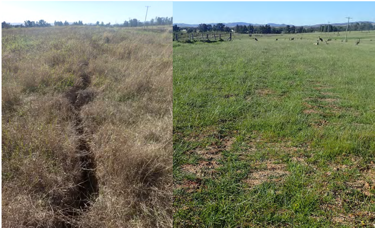
Photo 2: Example of subsidence cracking along stacked goaf edge and after crack remediation
