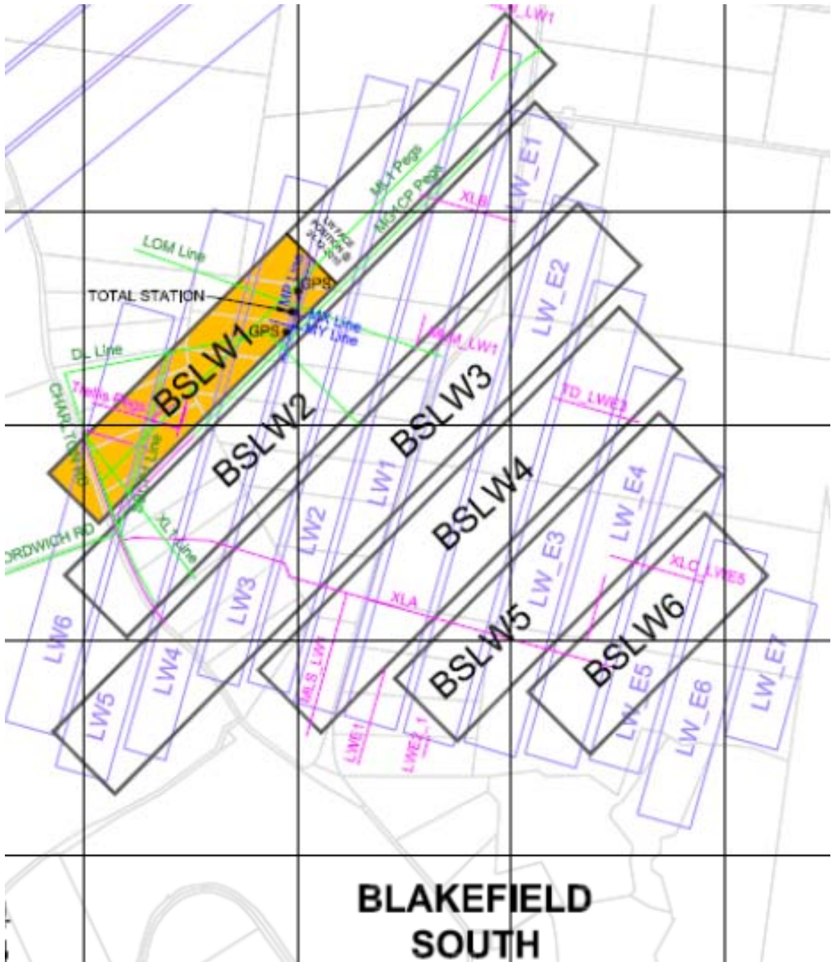
Fig. 4.19 Mine layout for Blakefield South Mine Longwalls 1 to 6 under the South Bulga Colliery Longwalls 3 to 6 plus the Locations of Various Subsidence Monitoring Lines
