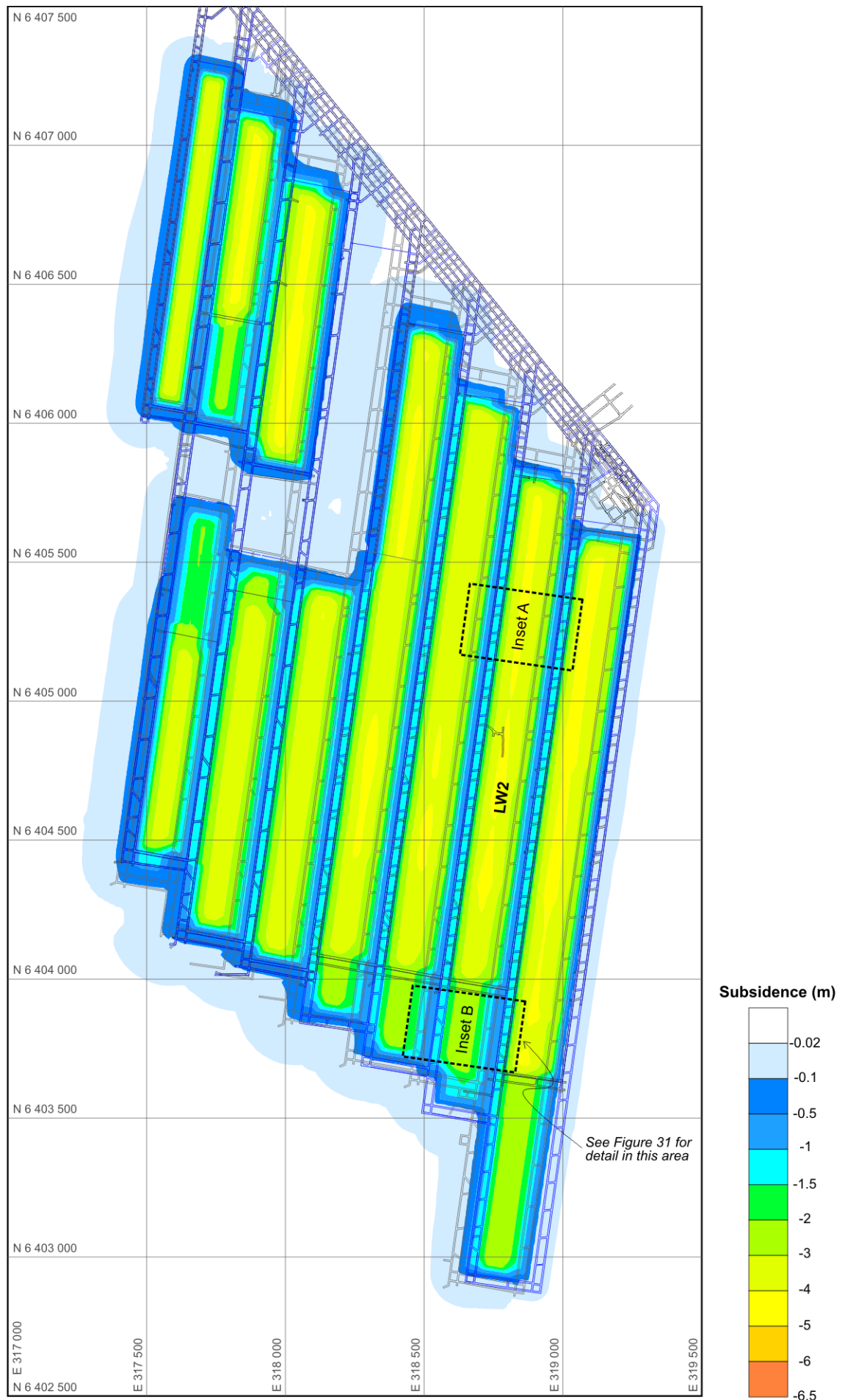
Figure 30: Cumulative Pike's Gully, Upper Liddell and Upper Lower Liddell Seam subsidence.
