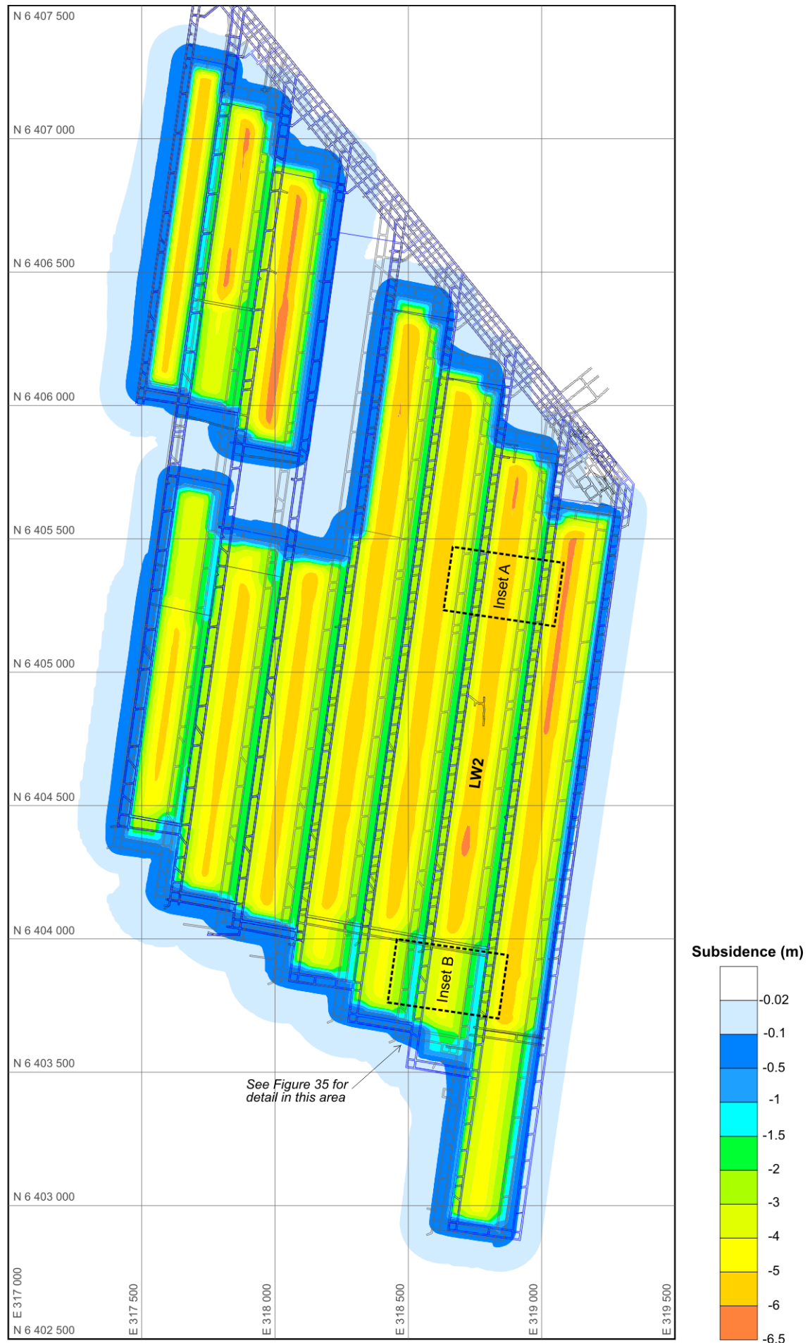
Figure 34: Cumulative Pikes Gully, Upper Liddell, Upper Lower Liddell and Lower Barrett Seam subsidence.
