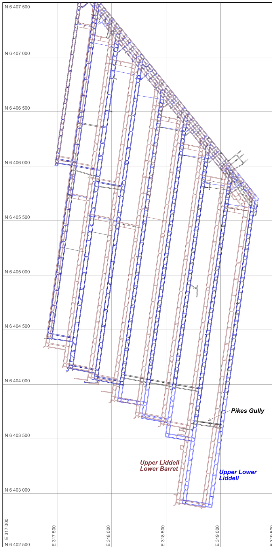
Figure 1: Pikes Gully, Upper Liddell, Upper Lower Liddell and Lower Barrett mine plans.
