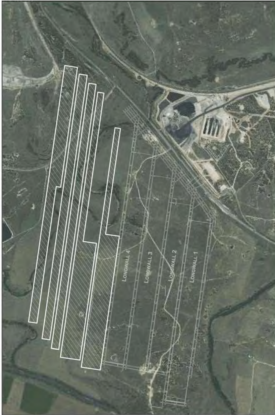
Figure 2 Longwall layout superimposed onto aerial photograph.
