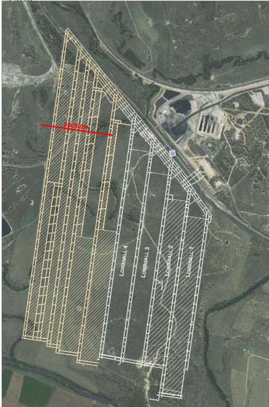
Figure 18(a) Approximate location for modelled cross-section of miniwalls 6-9 based on a width to depth of 0.6 with subcritical chain pillars designed to a Factor of Safety of 2.5.
