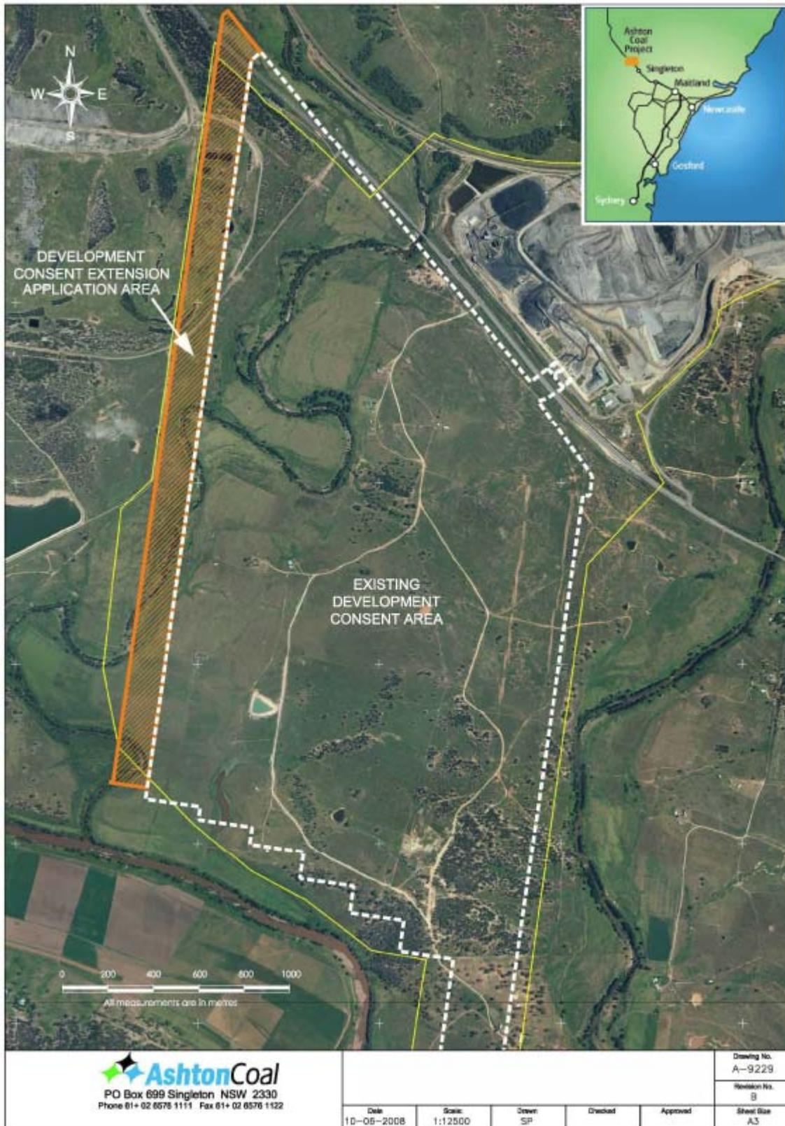
Figure 3: Area proposed for additional longwall mining
