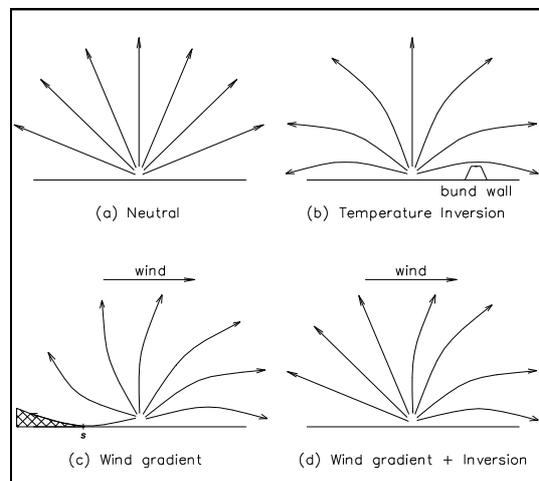
**Figure 1(b)** shows that sound rays can be refracted over a barrier (usually a bund wall or small hill) during a temperature inversion, greatly increasing noise levels in the ‘shadow zone’.
