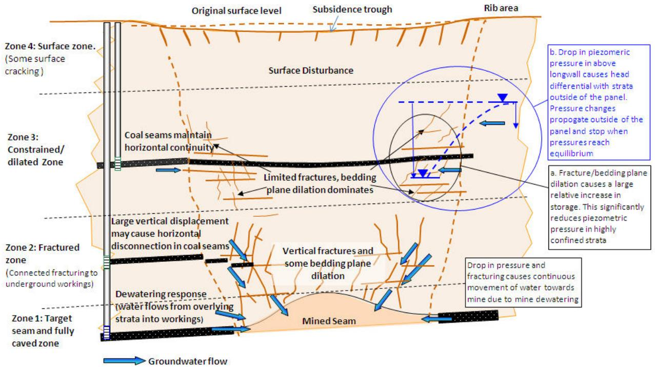
Schematic diagram showing mining induced disturbance zones
